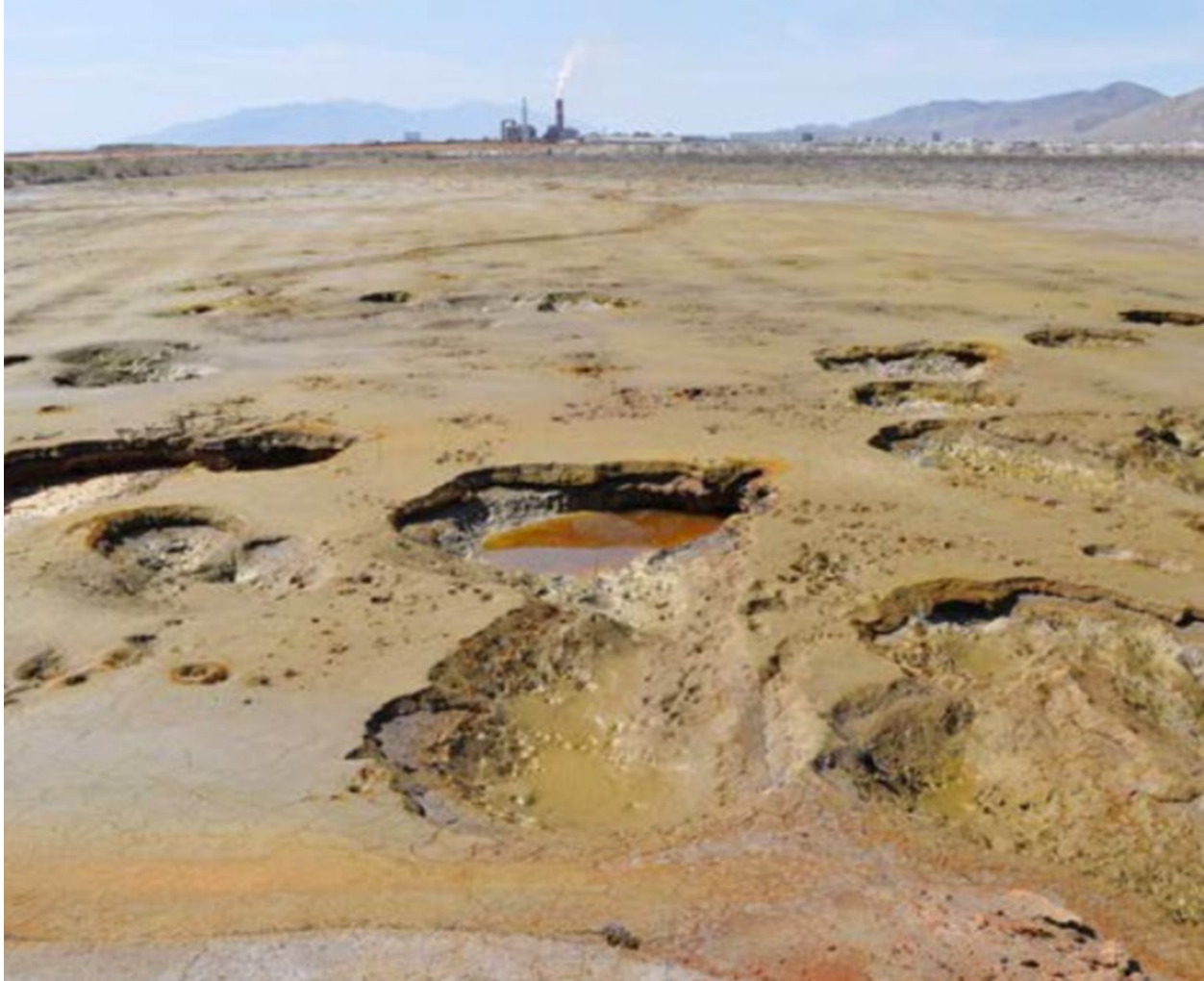
Figure 4. Image of dissolution channels observed as surface sinkholes in the bed of the active waste pond. US Magnesium plant is seen in the middle distance (looking south).
