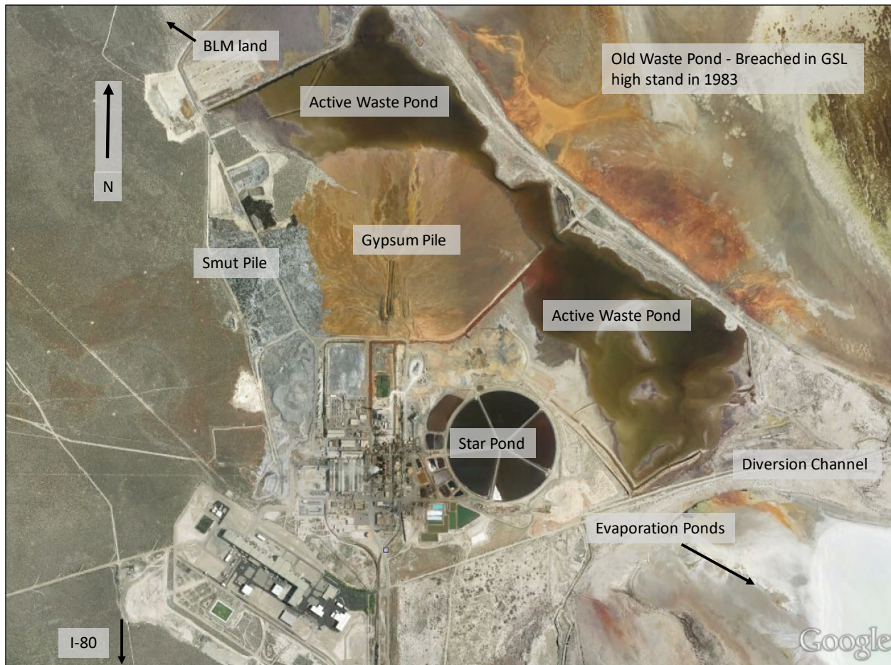
Figure 1. US Magnesium site layout showing Star Pond, Active Waste Pond, Gypsum Pile, Smut Pile, and Old Waste Pond.
